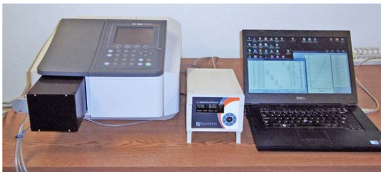
Figure 2. Testing the qCHANGER 6 with a Shimadzu UV-1800
