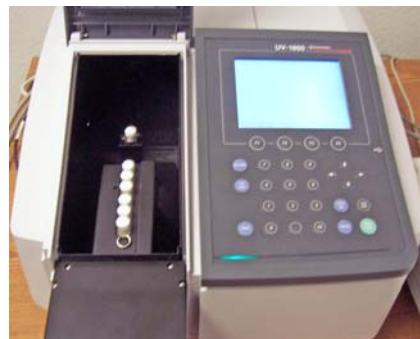
Figure 3. qCHANGER 6 mounted in the Shimadzu UV-1800
