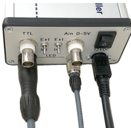
Figure 5: Cable connections on the back panel of the UHPTLCC LED current controller
