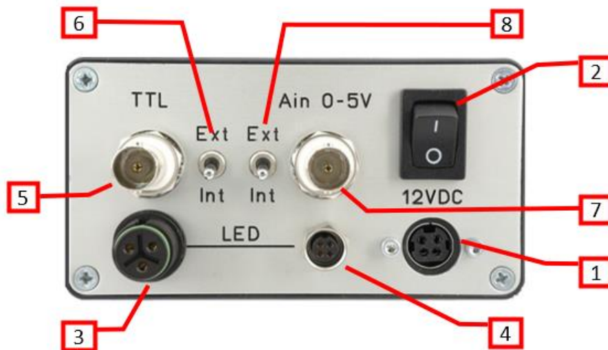
Figure 2: Back panel of UHPTLCC-02 Current Controller: (1) 12V DC power jack, (2) Power On/Off switch, (3) LED current cable connector (3 contacts) , (4) LED control cable connector (4 contacts), (5) TTL input connector, (6) TTL input enable toggle switch (external TTL input is enabled at “Ext” position), (7) Analog input connector, (8) Analog input enable toggle switch (external Analog input is enabled at “Ext” position).
