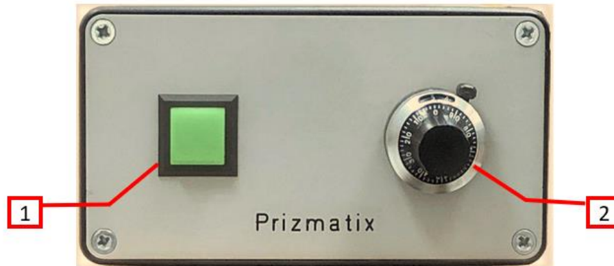
Figure 1: Front panel of UHPTLCC-02 Current Controller: (1) LED light On/Off switch with internal LED indicator, (2) Power adjustment dial (10-turn potentiometer).
