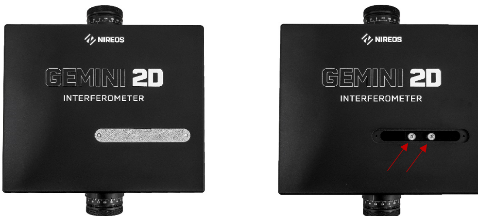
Figure 3: Pictures of the top of the GEMINI 2D, showing how to access the two mounts to fix the arrival time of the vertical replica during a scan of T_1 .
